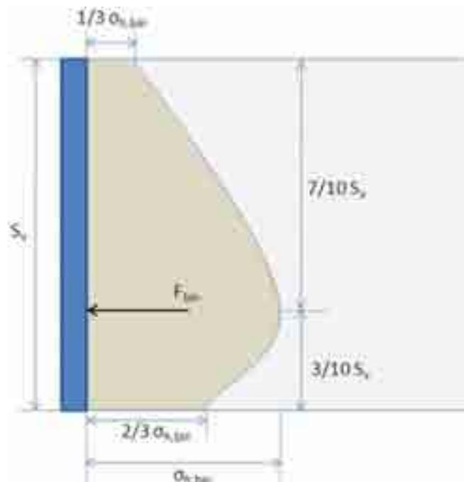
**Figure 10. Illustration. Bin pressure diagram for GRS structures.<sup>(11)</sup>**
