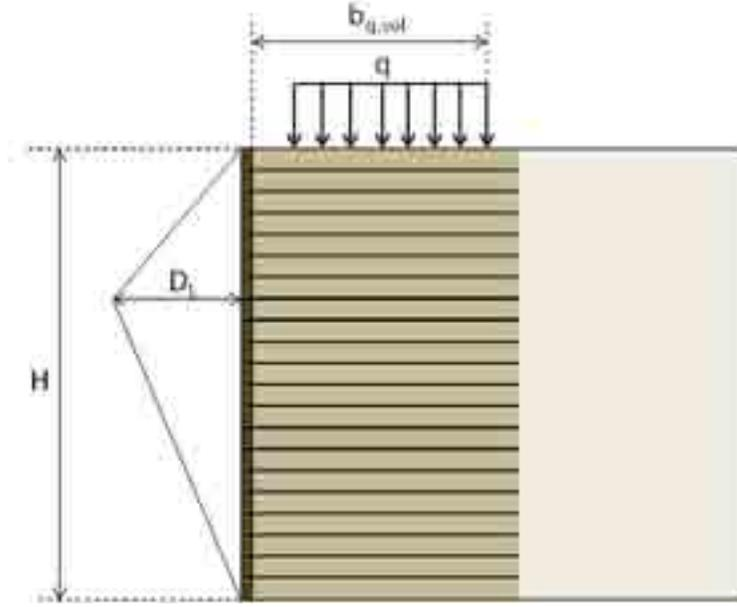
Figure 15. Illustration. Lateral deformation of a GRS structure.
