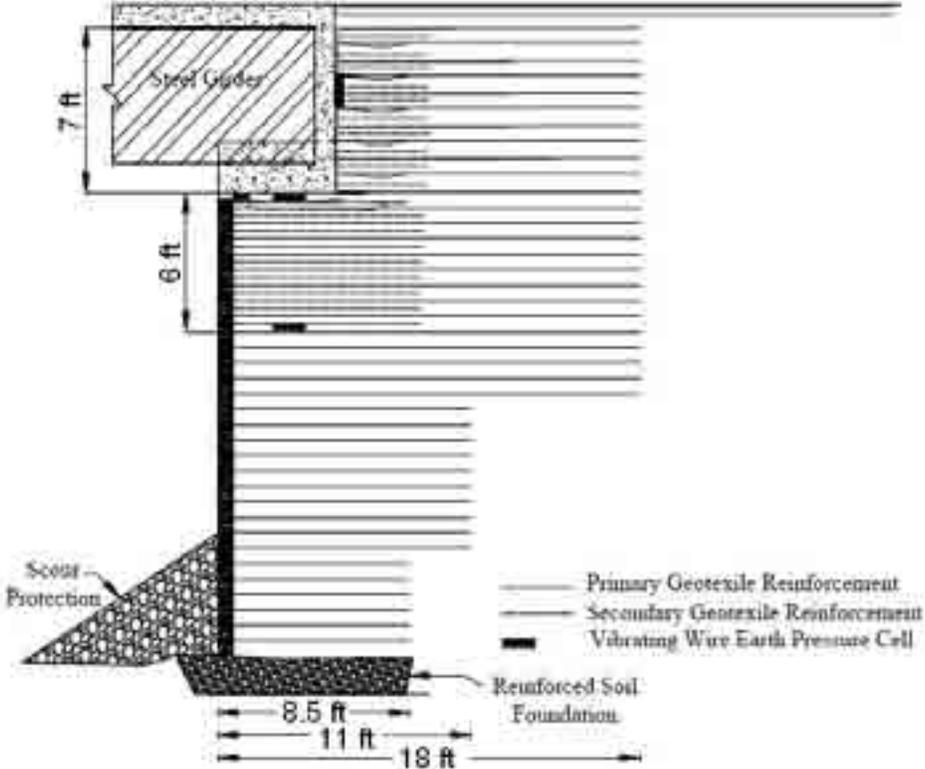
**Figure 38. Illustration. Instrumentation for Tiffin River Bridge.**
