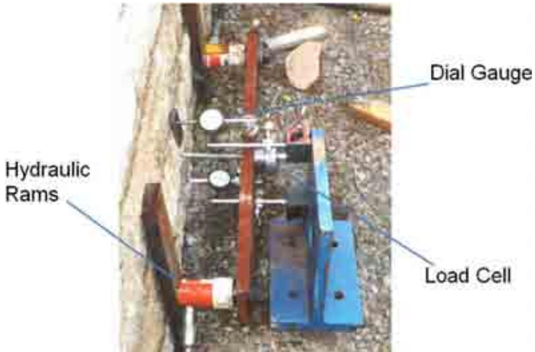
Figure 42. Photo. Block pull-out test on GRS wall.
