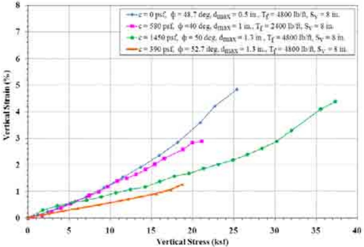
**Figure 11. Graph. Performance test results for different materials.**
