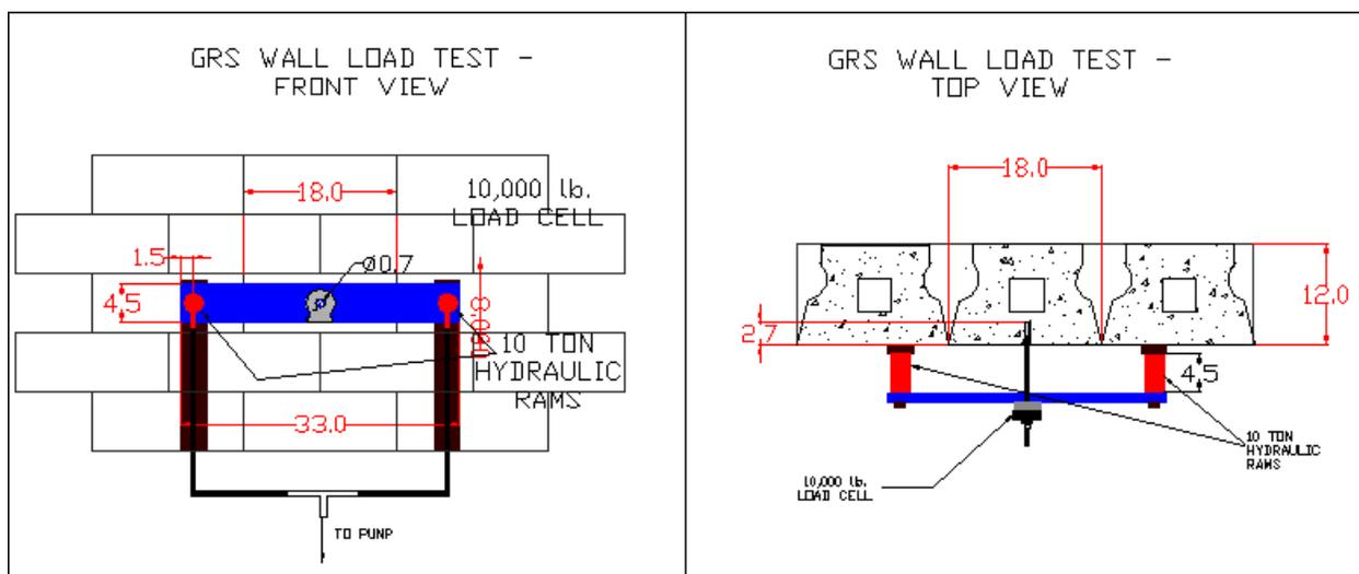
Figure 43. Illustration. Block pull-out test setup.
