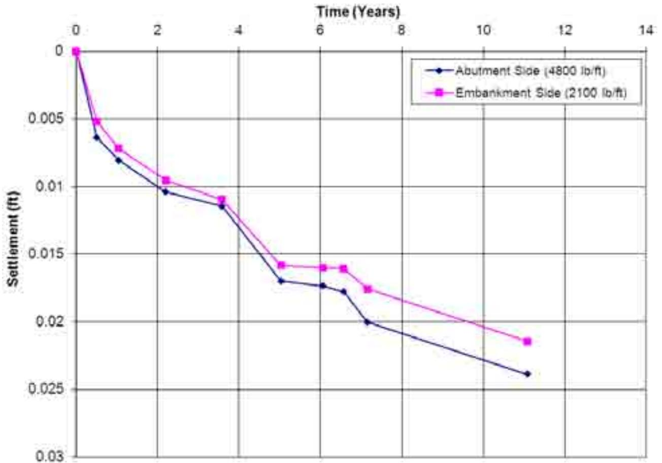
**Figure 30. Graph. Settlement versus time for TFHRC tunnel.**
