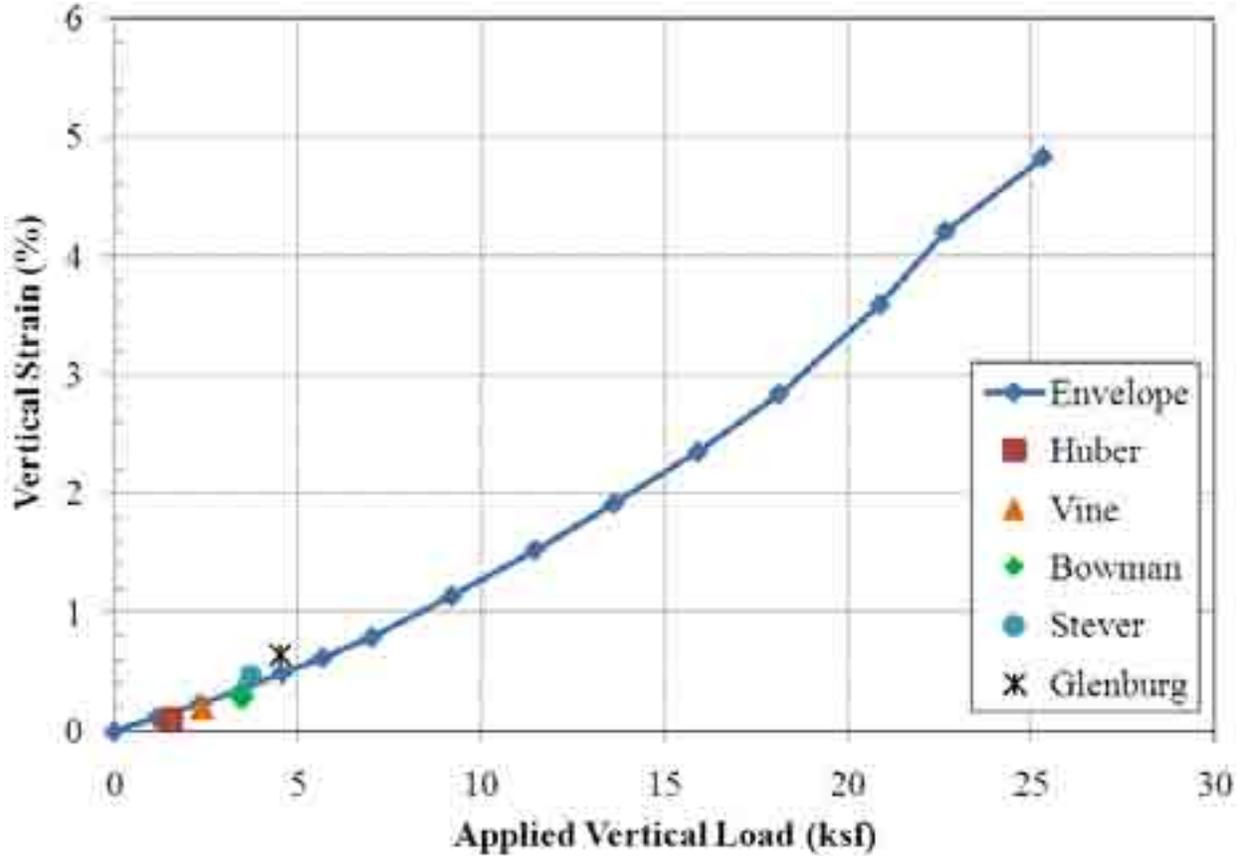
Figure 14. Graph. Deformation estimation from in-service GRS-IBS structures.
