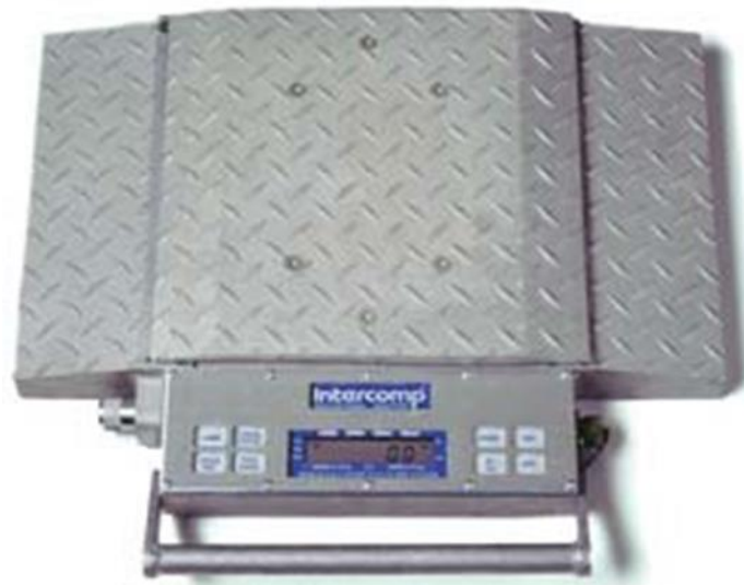
Figure 4.5: Wheel Load Weigher (Intercomp)
