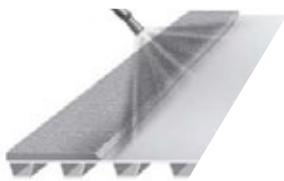
2 Weld perimeter bars to deck and weld top plate to form air-tight cavities
