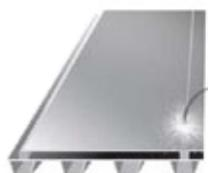
3 Inject elastomer into cavities and allow to cure
