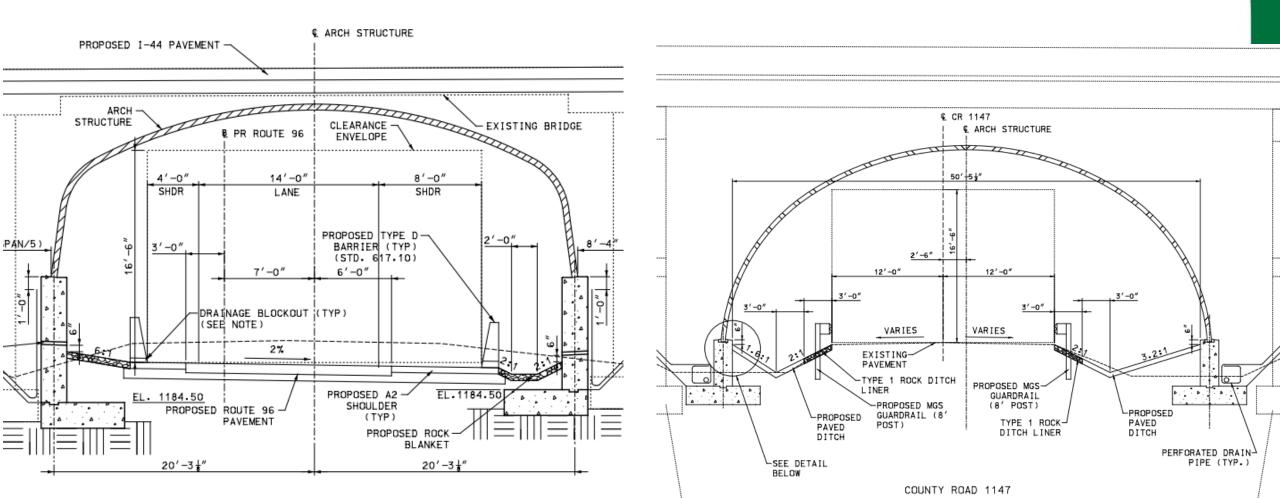
Customized layouts & end treatments to accommodate site configurations: Rte 96 – unbalanced step bevel to address skewed alignment with I-44
