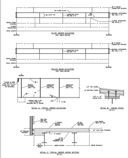
DESIGN DATA SHEET USAGE THESE DESIGN DATA SHEETS PROVIDE PRELIMINARY STEEL BEAM SIZING AND DETAILING INFORMATION FOR THE LENGTHS, GIRDER SPACINGS, LOADINGS, AND OTHER DESIGN CRITERIA NOTED HEREIN, DEVIATIONS FROM THE CRITERIA INCORPORATED HEREIN MAY NECESSITATE MODIFICATION TO GIRDER SIZES. IT IS THE RESPONSIBILITY OF THE ENGINEER OF RECORD TO ASSURE ADHERENCE TO STATE AND FEDERAL
