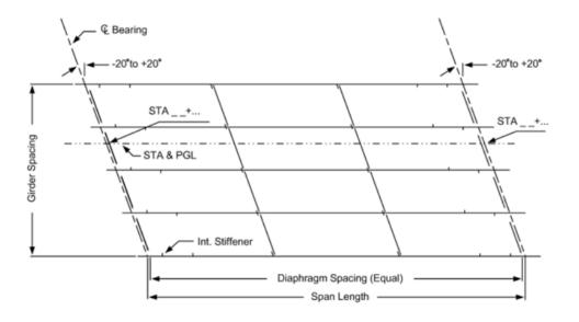
Example output (sample plate girder elevation):
