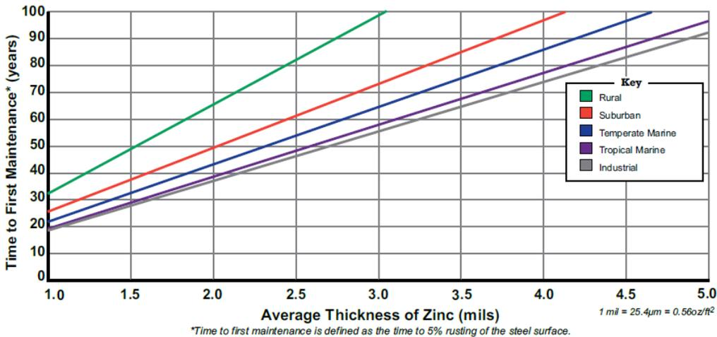
**Figure 3: Time to First Maintenance for Hot Dip Galvanized Bridges<sup>3</sup>**
