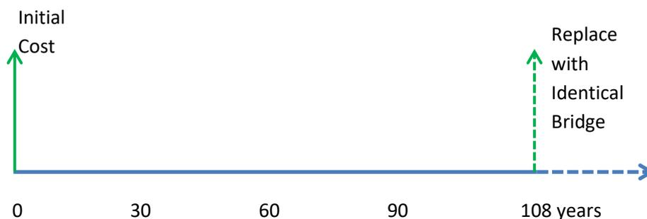
**Figure 5: PennDOT Galvanized Bridge 6520 Life Cycle Cost Timeline**
